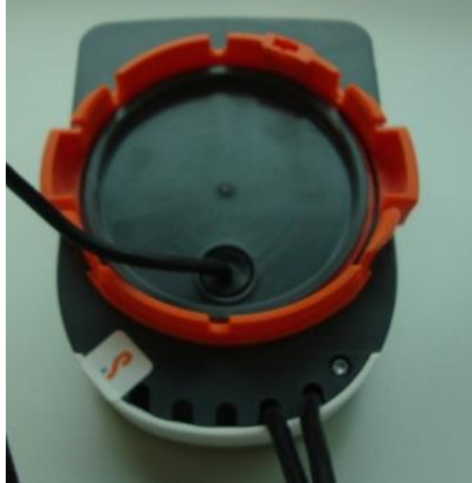
Figure 7 – Securing of the calculator by means of a sticker
