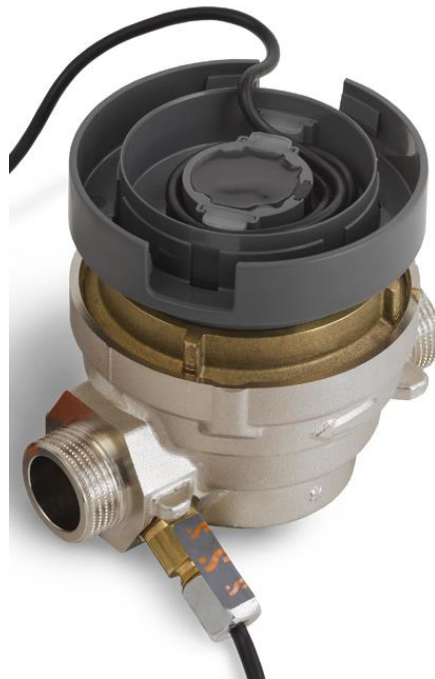
Figure 6 – Flow sensor (multi-jet measurement capsule meter) can't be removed non-destructively and the temperature sensors are sealed by stickers
