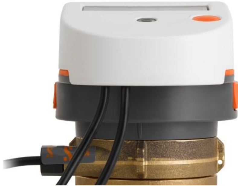
Figure 5 – Flow sensor (multi-jet measurement capsule meter) can't be removed non-destructively and the temperature sensors are sealed by stickers
